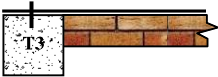
Outside face (including frame elements) strengthened with CFRP
