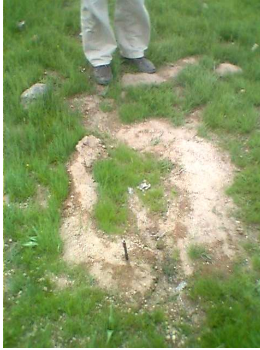
Figure 4.28 Sand boil at Hanoçayırı (Point 16 in Figure 4.13) (N 390 03.1', E 400 30.46')
